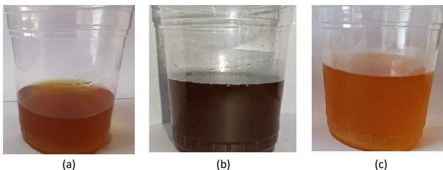
**Figure 6.** The color of rice straw extract: (a) soxhlet, (b) reflux, and (c) maceration
