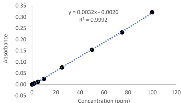
Figure 3. Standard Curve of TFC Analysis
