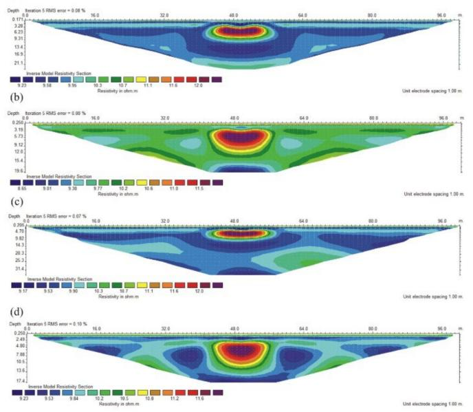
Figure 5. Inverse models of (a) Dipole-Dipole, (b) Wenner-Schlumberger (c) Pole-Dipole and (d) Wenner arrays.
