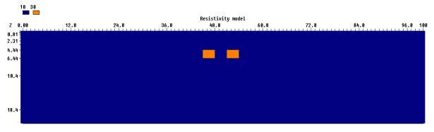
Figure 3. The 2D synthetic model of two structures separated by a distance of 3m.
