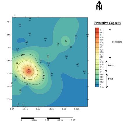
Figure 16. Longitudinal Conductance (Ohms<sup>-1</sup>), Map of the Study Area.
