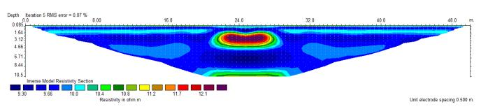
Figure 6. Inverse models of dipole-dipole array with 0.5m electrodes spacing for two structures separated by a distance of 3m.
