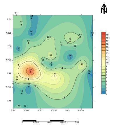
Figure 15. Layer thickness above the aquifer (meters).
