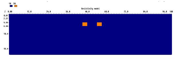
Figure 4. The 2D synthetic model of two structures separated by a distance of 6m.
