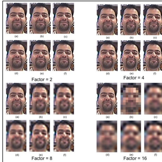
Fig. 8: Different qualities were observed on each magnification factor for the common resizing method against (f) Sparse Representation SR - (b) Nearest Neighbor, (c) Bicubic, (d) Bilinear, (e) Lanczos. (a) Here is the ground truth tested on the UKM-CSM Dataset.
